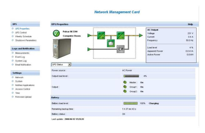
These measurements are available for AC to DC converter, Battery, DC to AC converter and automatic bypass. The measurements available in these boxes depend on the UPS range.
